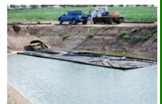
13. Demonstration cover, 16 x 8 m, floating on the pond and being inflated to simulate gas capture - demonstrates 'proof of concept'. Unfortunately this was taken after the MINTRAC visit.
